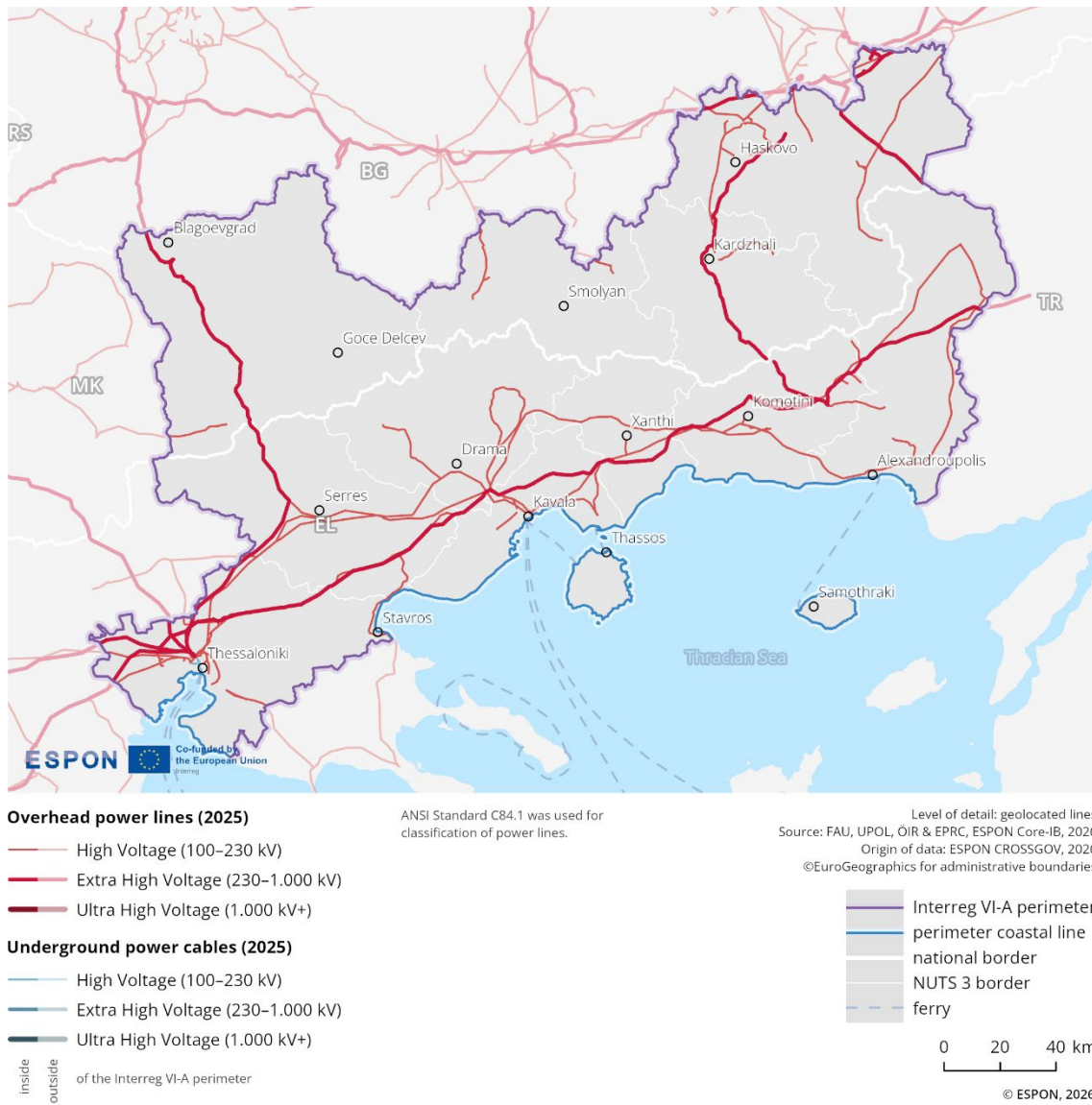
Figure 2.23: High-voltage transmission infrastructure
