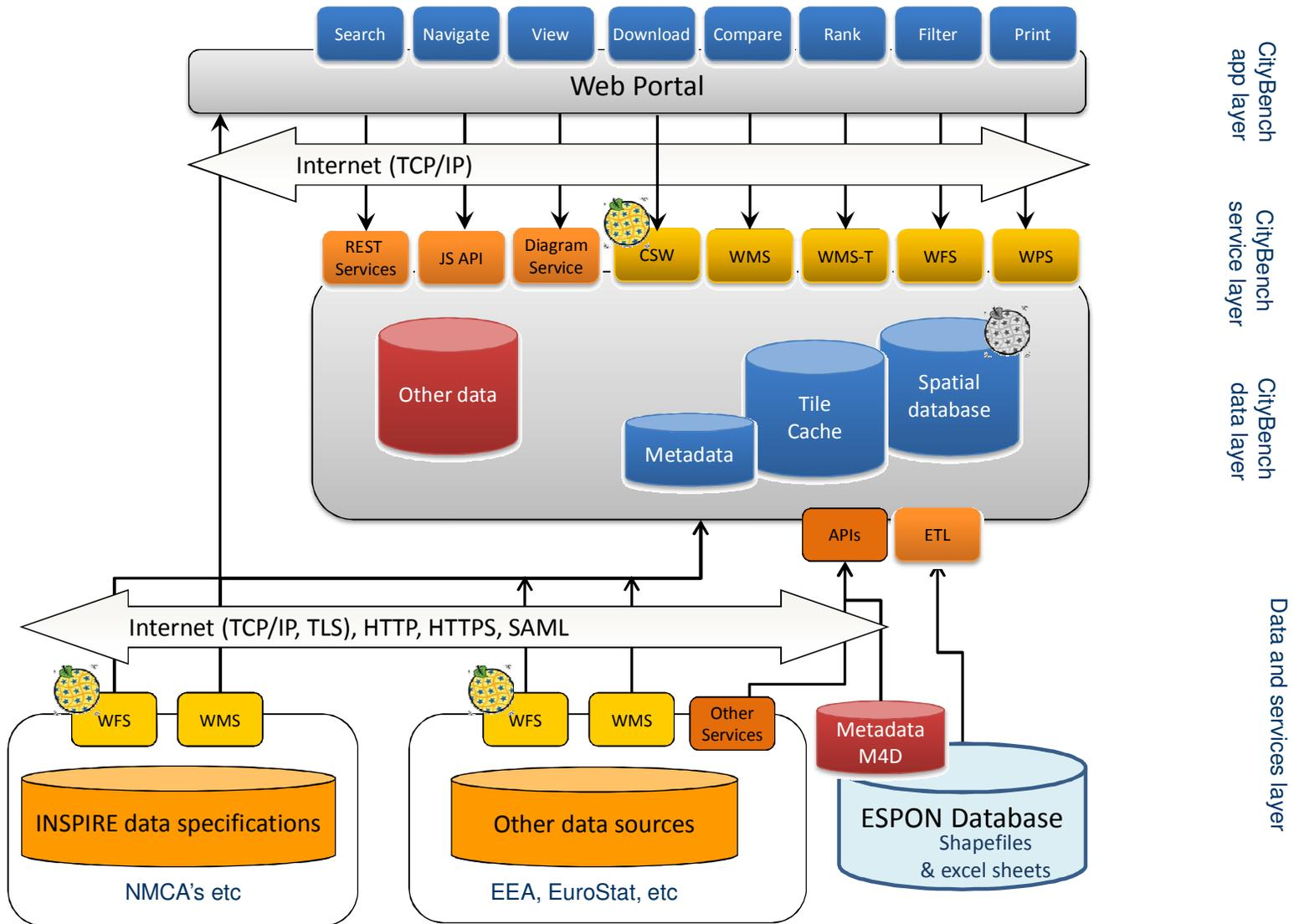
Figure 9 – CityBench conceptual Architecture
