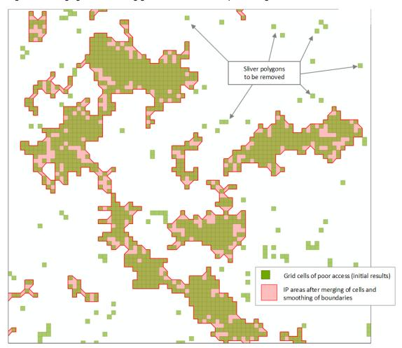
Figure 3.4. Merging and smoothing grid cells before further processing.
